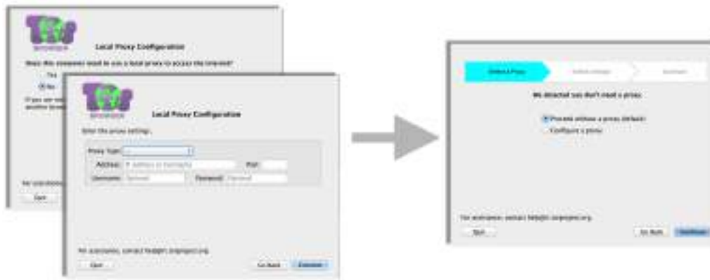
Fig. 5. In the OLD interface, users are asked, “Does this computer need a local proxy to connect to the Internet?” (P1). A “Yes” determines that a proxy should be configured and directs to the proxy configuration screen (P2). The NEW interface checks the local machine’s proxy settings, and informs the user whether a proxy is required, and if so, what those settings are (P).
