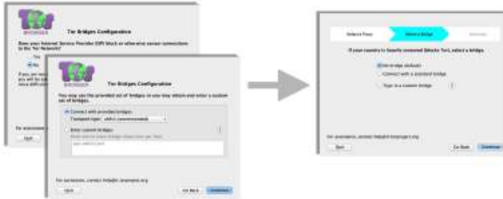
Fig. 4. In the OLD interface, users are asked, “Does your Internet Service Provider (ISP) block or otherwise censor connections to the Tor Network?” (B1). A “Yes” determines that a bridge should be configured and directs to the bridge configuration screen (B2). The NEW interface gives users advice on configuring bridges while giving the option of not configuring a bridge, on one screen (B).
