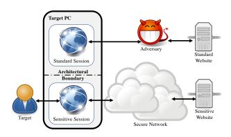
Figure 2: Remote cache-based website fingerprinting attack model. The remote attacker injects malicious JavaScript code into a browser running on the target machine.
